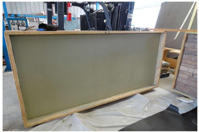
SUBSTRATE: AIR & WATER BARRIER / ½" CEMENT BOARD SHEATING / 2x4 WOOD FRAMING
