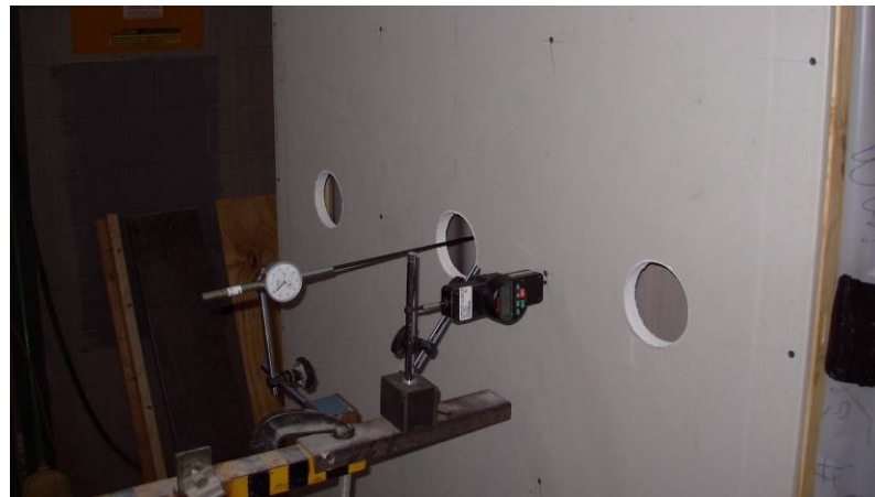
Gage locations on test wall assembly. One gage on back of wall assembly and one gage on back of plywood/fiberglass gypsum sheathing
