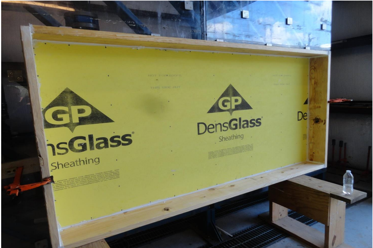
½" DENSGLOSS SHEATHING FASTENED TO STEEL FRAMING
