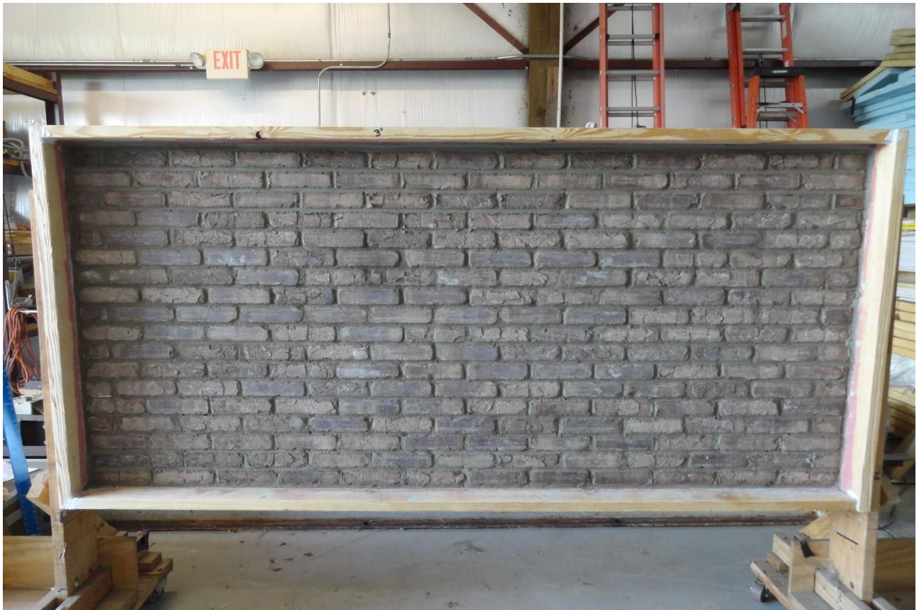
FINAL THIN BRICK WALL ASSEMBLY
