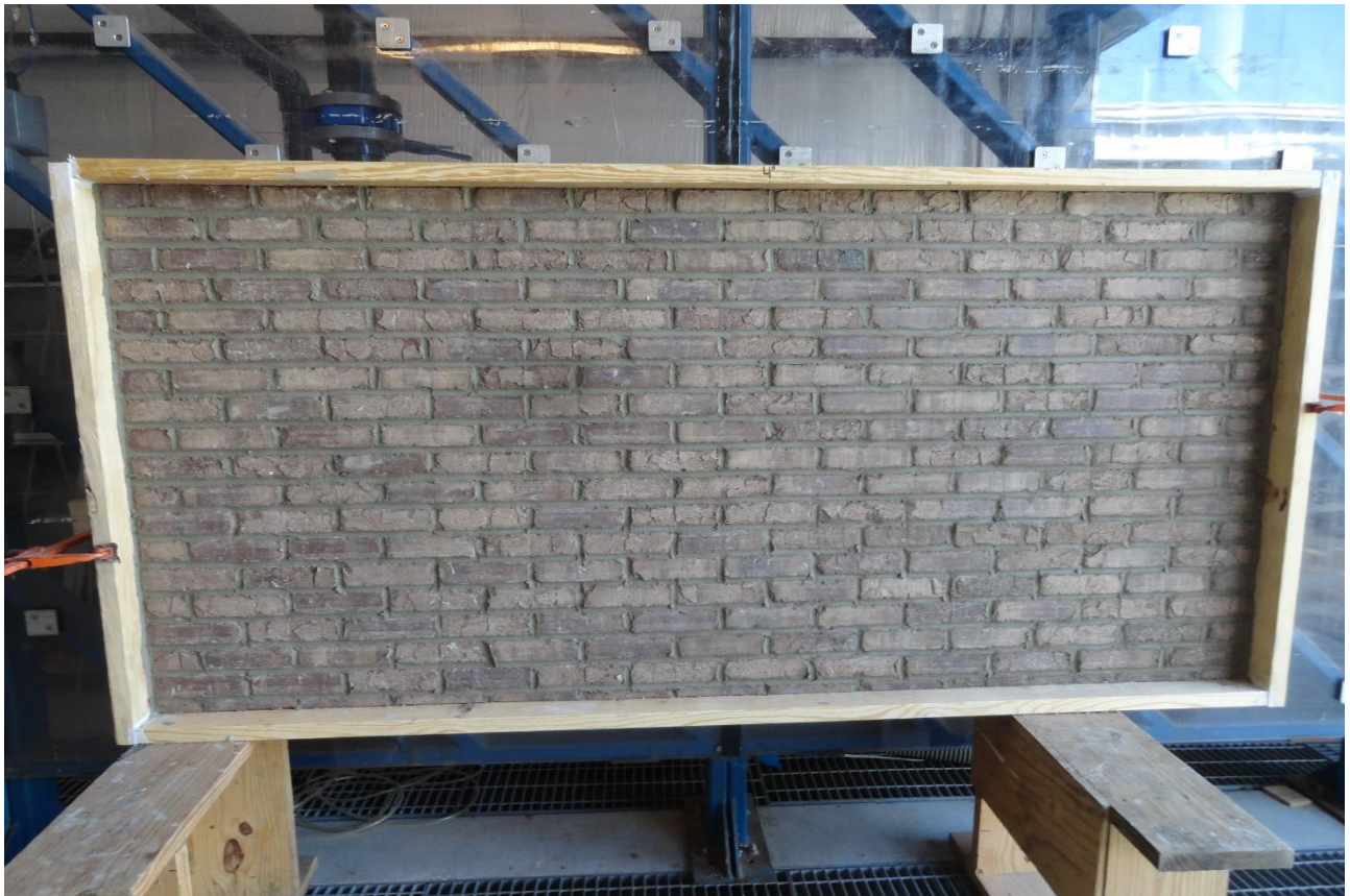
FINAL THIN BRICK WALL ASSEMBLY
